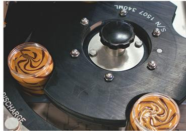
NUT BUTTER ROTARY VOLUMETRIC FILLER
